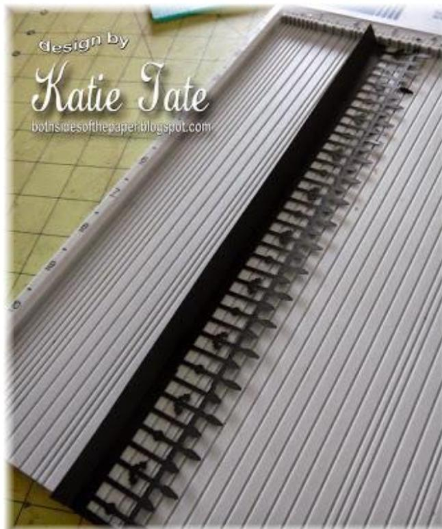
Punch a 12" strip with your fence punch from a full piece of cardstock. After punching trim to a height of 2" on a trimmer. Then on your Scor-Pal score a line 1/4" from the bottom of your fence and burnish. These measurements will vary depending on what you use for your fence. Just remember that you need to leave room to be able to form a flap that will attach to the base.
